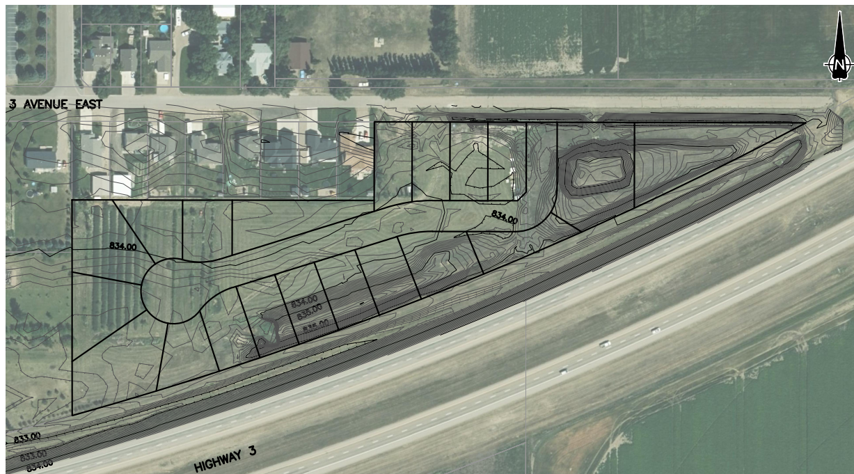
Figure 2: Existing Site Topography
